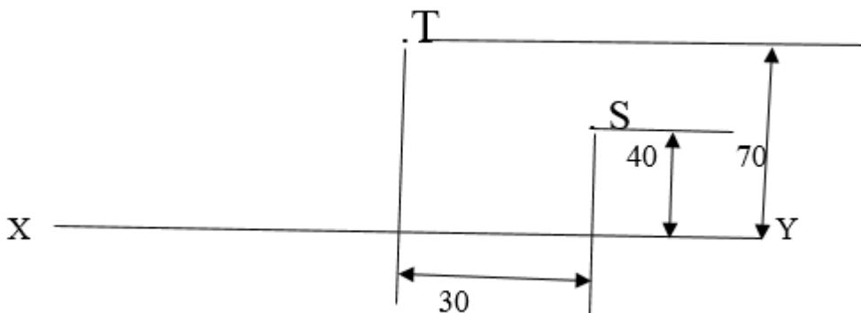
i. Construct a circle to touch line XY and pass through point T and S (7 marks)
